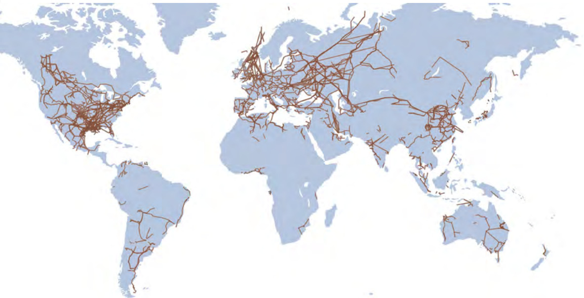
Figure 4.3 Global map of natural gas transmission pipelines
